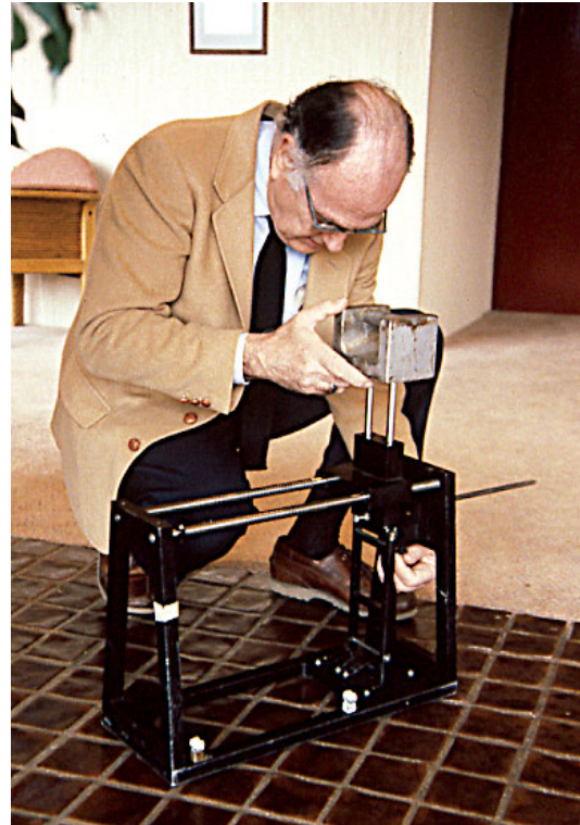
A tribometer for evaluating slip resistance. (Photo courtesy of Jake Pauls)
