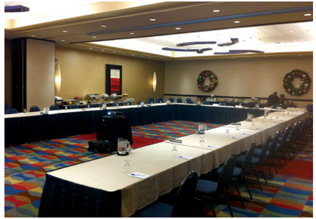
Meeting room setup for fewer than 50 persons not constituting an assembly occupancy.
