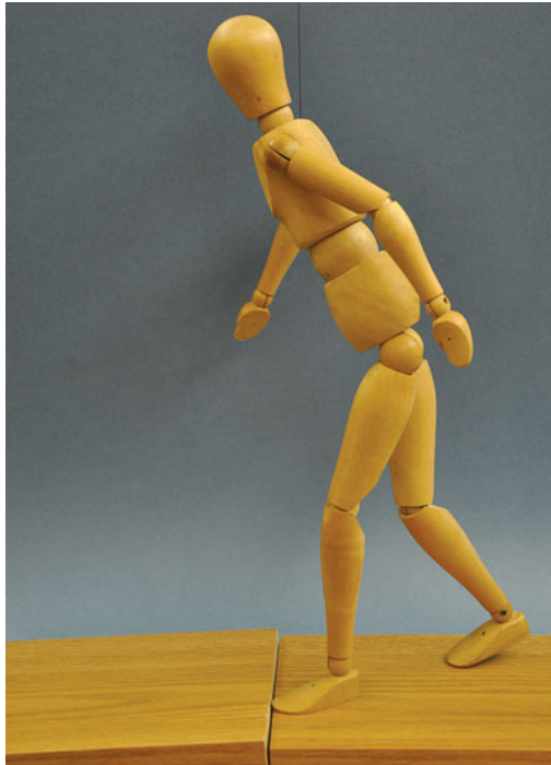
Simulation of foot contacting small elevation difference in walking surface. (Photo courtesy of Jake Pauls)
