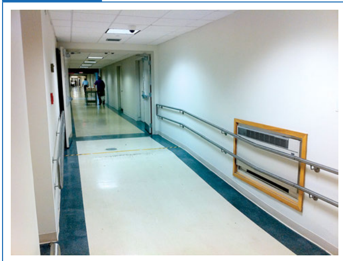
Indoor ramp for small elevation change between building sections.
