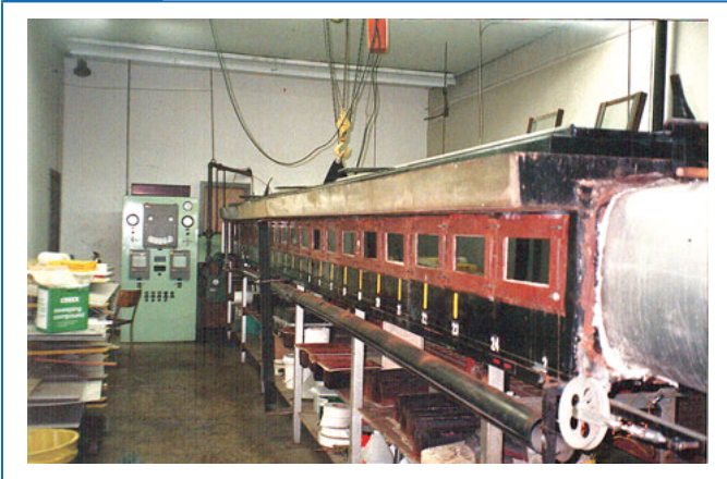
ASTM E 84 room tunnel test apparatus. (Photo courtesy of Herbert Blenstein)
