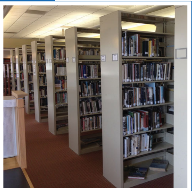
Library stack area for which Code specifies an occupant load factor of 100 ft 2 (9.3 m 2 ) per person.
