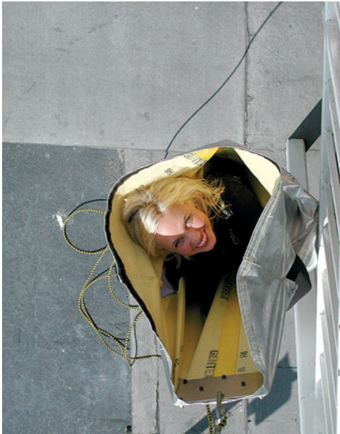
Evacuee inside protective suit while using controlled descent device. (Photo courtesy of High-Rise Escape Systems, Inc.)
