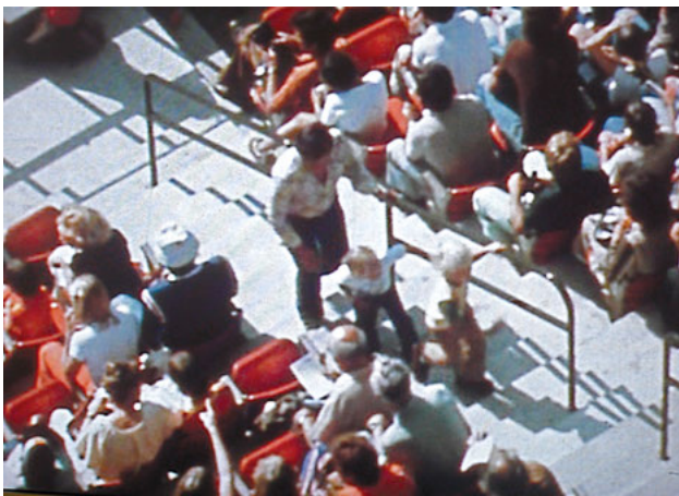
Field testing of handrail height. (Photo courtesy of Jake Pauls)
