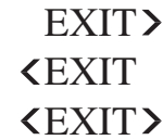
FIGURE A.7.10.6.2 Directional Indicators.
