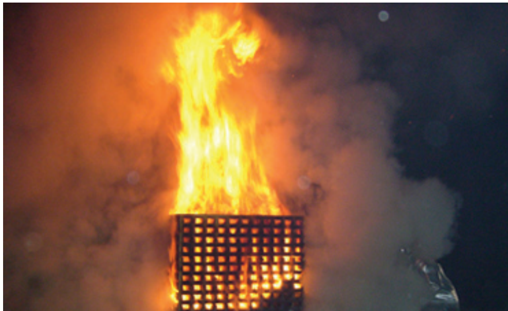
Exhibit 6(a) 10-A Wood Crib Fire Test. (Photo courtesy of Amerex Corporation)
