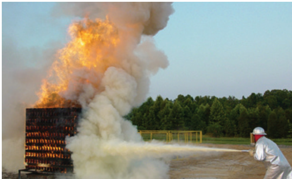
Exhibit 6(b) 30-A Wood Crib Fire Test. (Photo courtesy of Kidde Fire Protection/United Technologies Corp.)
