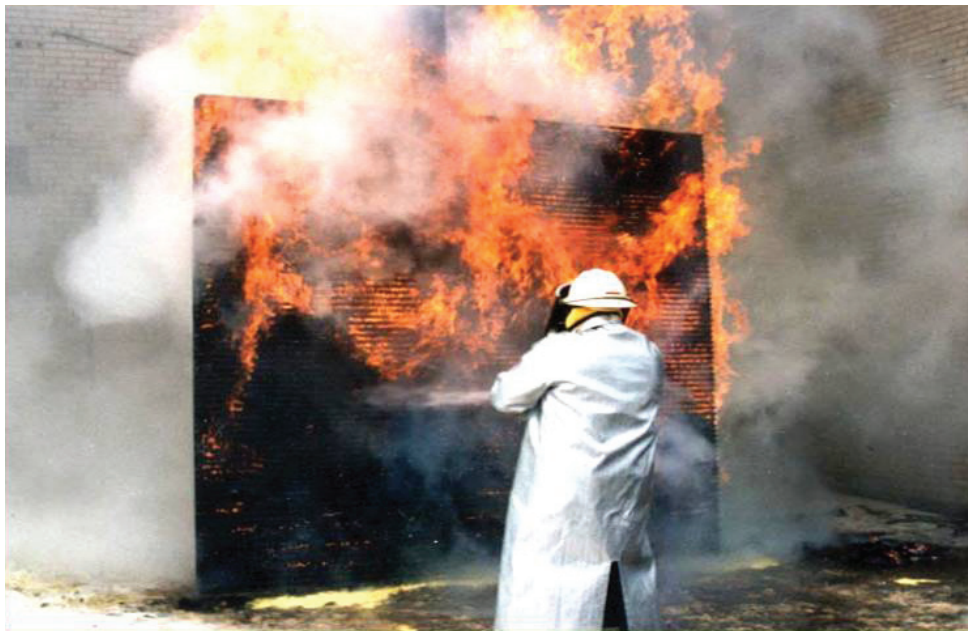
Exhibit 7 Wood Panel Fire Test. (Photo courtesy of Amerex Corporation)
