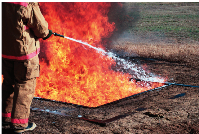
Exhibit 8 Class B Fire Test. (Photo provided courtesy of Amerex Corporation)
