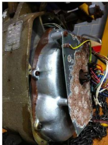
Corrosion inside the cover of an electric chain hoist
