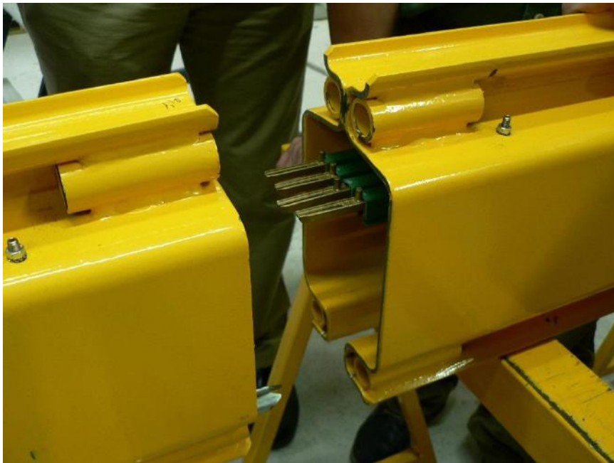
Steel Profile Connection Bolts with Internal Power Conductor System Connection Joint
