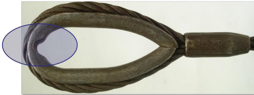
Damaged Reeving Thimble
