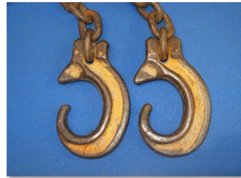
'C' Hooks (designed to be used without safety latches)
