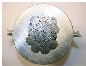
Cross- Section of a Pressed Ferrule Termination
