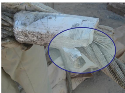
Cracked and Split Ferrule
