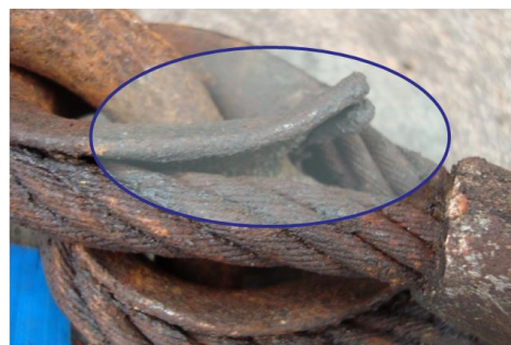
Damaged Thimble (Side Loading)
