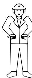
EXTEND BOOM (Telescoping Booms). Both fists in front of body with thumbs pointing outwards.
