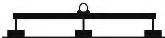
Figure 26.6 Support flexible loads with two or more magnetic lifters in conjunction with a lifting beam
