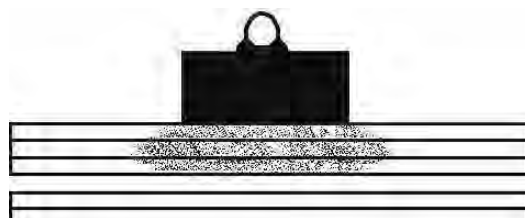
Figure 26.7 Magnetic lifters with variable power facilitates shedding of excess load
