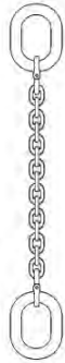
Figure 14.2 Collar sling (If one end will pass through the other, this is known as a reeveable collar sling)
