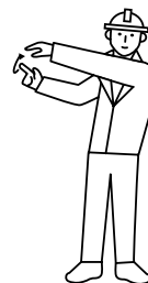
MOVE SLOWLY. Use one hand to give any motion signal and place other hand motionless in front of hand giving motion signal. (Hoist slowly shown as example.)
