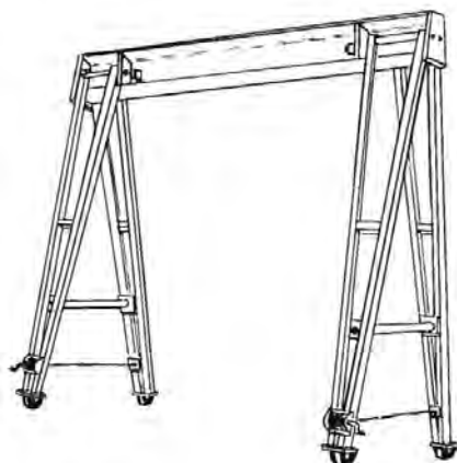
Figure 12.11 Self erecting gantry
