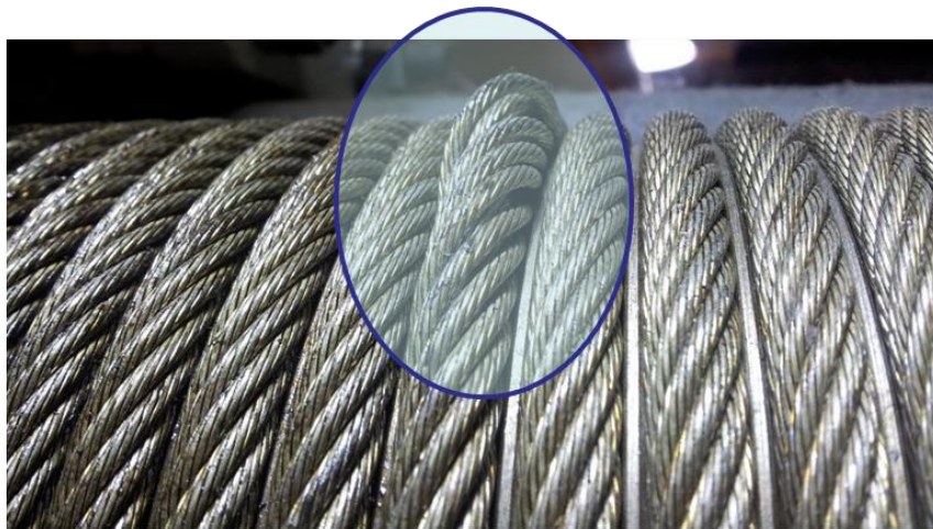
Damage to load rope from shock-loading
