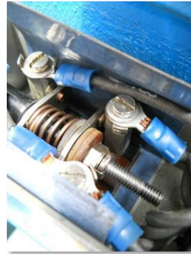
UP limit circuit "closed"
