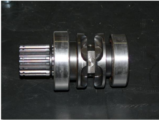
Load chain pocket wheel typically found in the electric chain hoist
