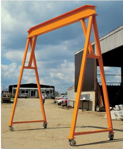
Internally Braced Gantry
