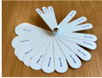
Sheave gauges measure wear on a sheave
