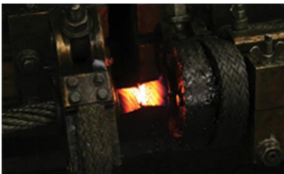
3. Rope Twisted Until it Parts
