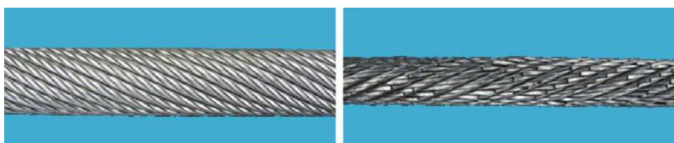
Figure B.4 — Complete rope shown on left and same rope with outer strands removed shown on right. Illustrates absence of external wire breaks, but presence of internal wire breaks
