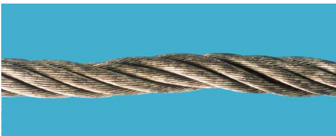
Figure B.5 — Local reduction in rope diameter (sunken strand)
