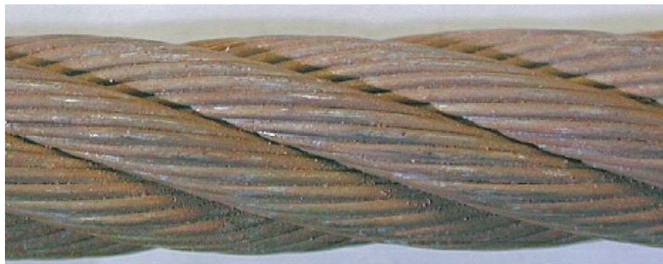
Figure I.1 — Beginning of surface oxidation, can be wiped clean, superficial — Rating: 0 % towards discard
