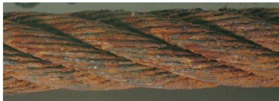
Figure I.3 — Surface of wire now greatly affected by oxidation — Rating: 60 % towards discard
