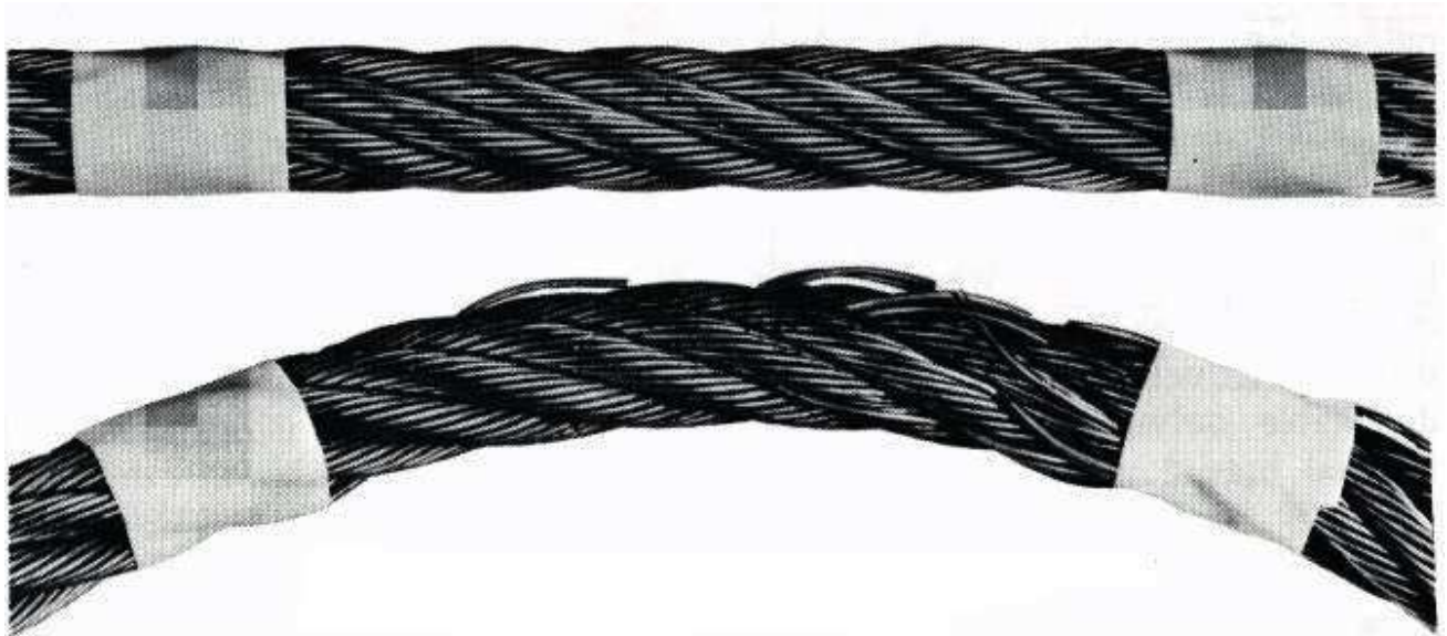
Figure 8 — Flexing a rope can often expose broken wires hidden in valleys between strands
