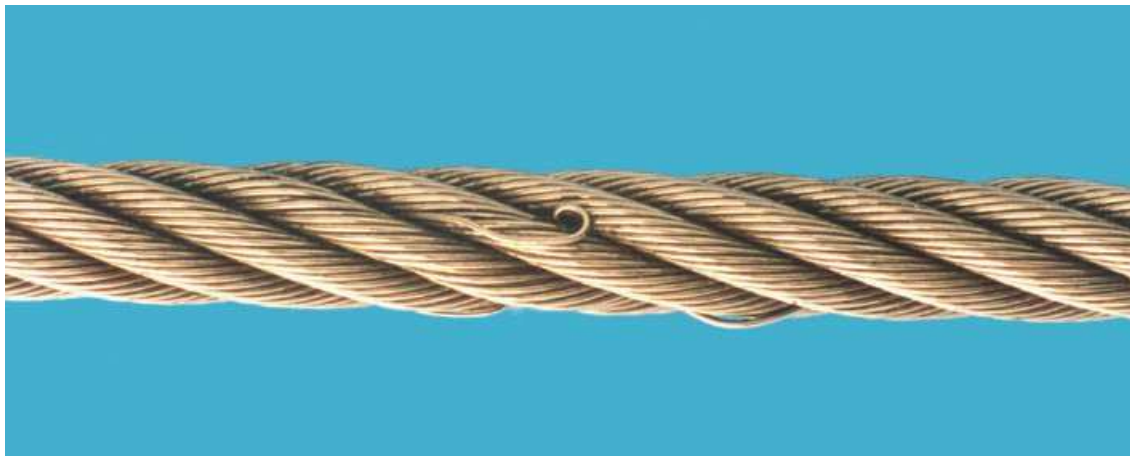
Figure B.14 — Wire protrusion
