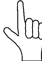
Start rope at left hand flange for left hand lay rope.
