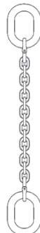
Figure 14.2 Collar sling (If one end will pass through the other, this is known as a reevable collar sling)
