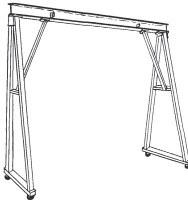
Figure 12.8 'A' frame mobile supporting structure
