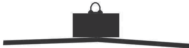
Figure 26.5 Beware of flexible loads peeling off the magnet face
