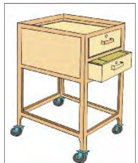
Figure 6e. An easy-to-move tool cart provides orderly storage and protection of tools and instruments.
