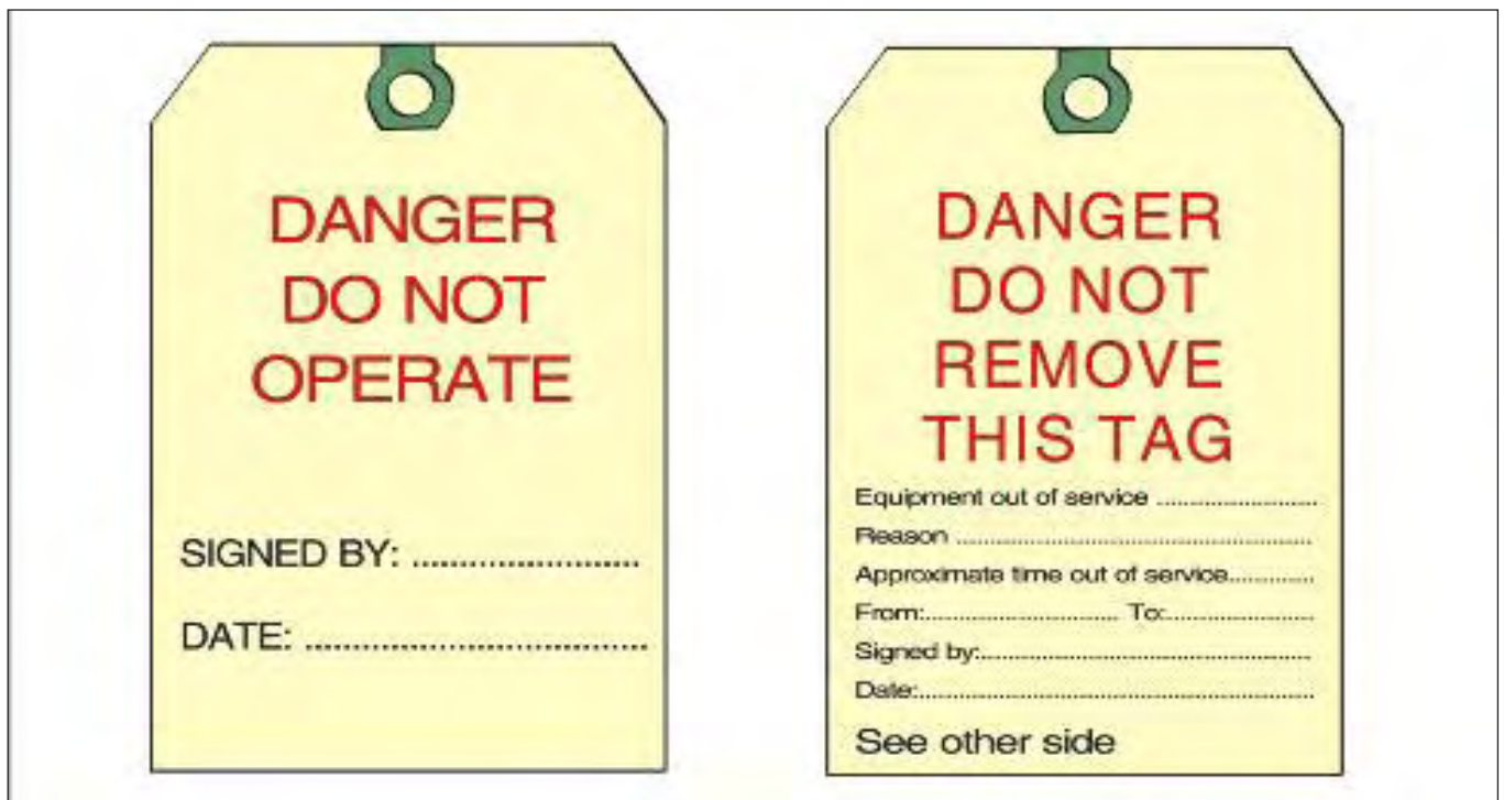
Figure 50a. Front and back views of a typical tag used when equipment is taken out of service because it has become unsafe.
