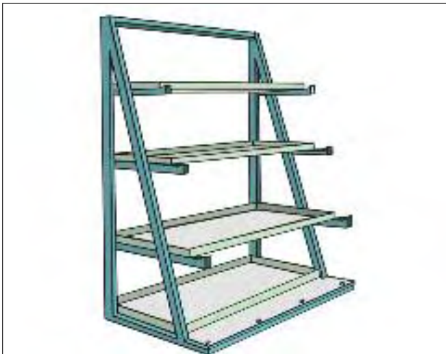
Figure 8c. A vertical rack. Metal rods and bars of different profile can be stored efficiently in a limited area or near the job. Tray-type shelves provide room for small pieces.
