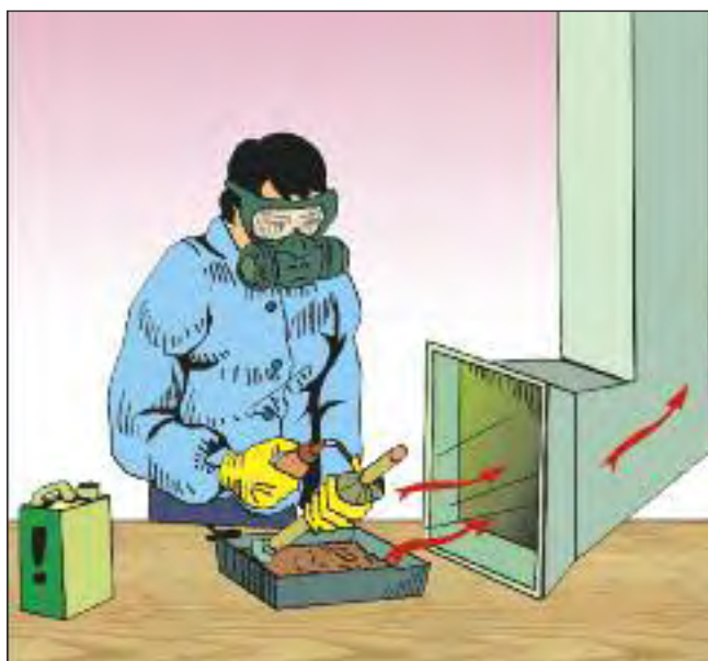
Figure 92a. Noxious fumes can be drawn into a local exhaust system to prevent the worker being exposed to chemical hazards.
