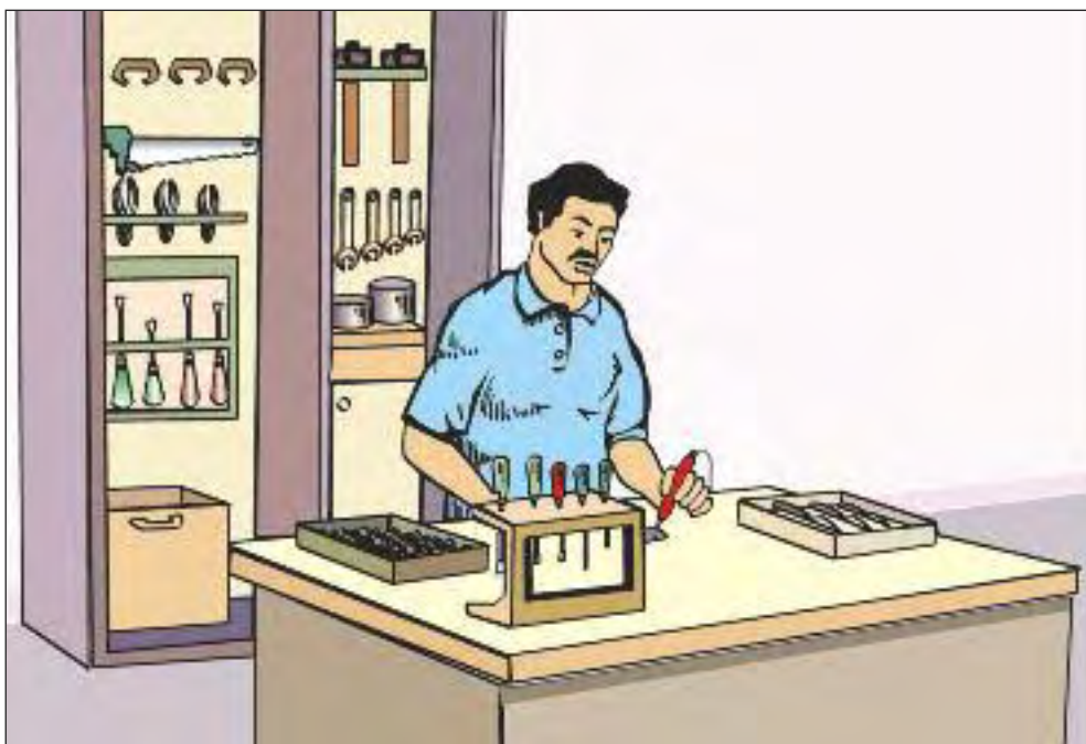
Figure 28c. Provide “homes” close to the worker for tools used repeatedly. “Homes” for tools used less frequently can be placed around the workstation.
