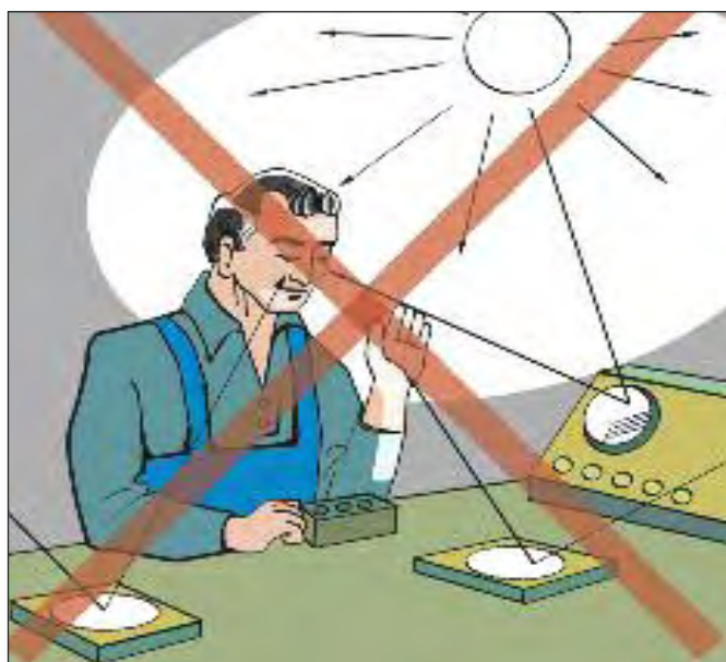
Figure 70c. Reflected (indirect) glare reduces visibility.
