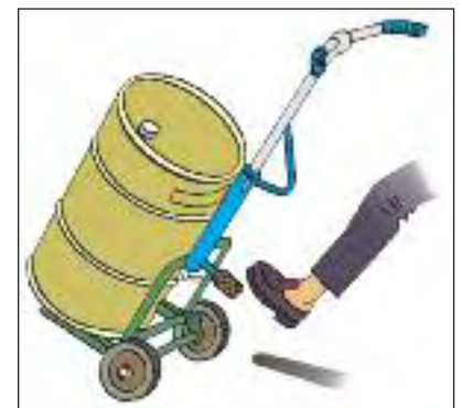
Figure 6c. This barrel-handling device not only makes work much easier but also helps avoid damage.
