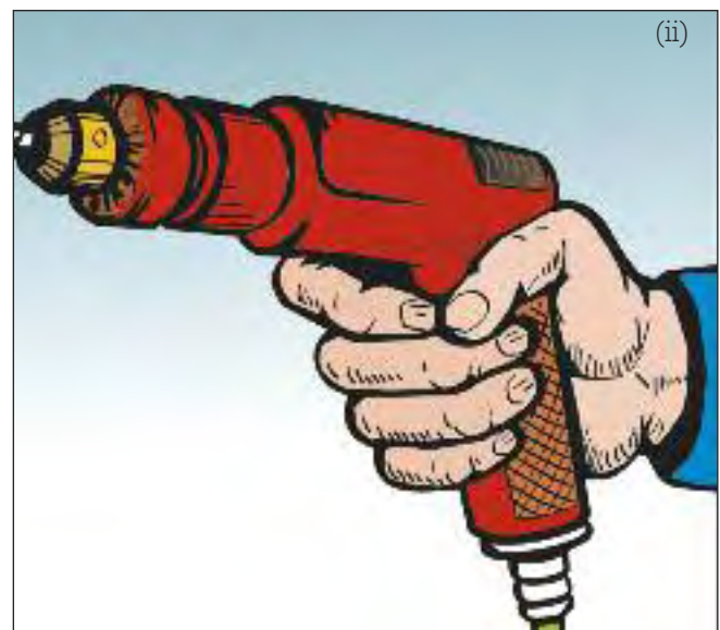
Figure 18c. (i) and (ii) Steady grips of power tools help reduce the required force of operation.
