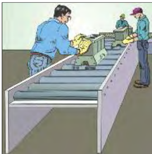
Figure 13c. Push and pull heavy materials instead of raising and lowering them.
