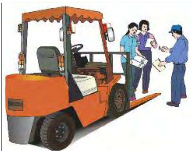
Figure 49b. Use a checklist to ensure the key safety features of forklifts and travel routes are operational before daily use.
