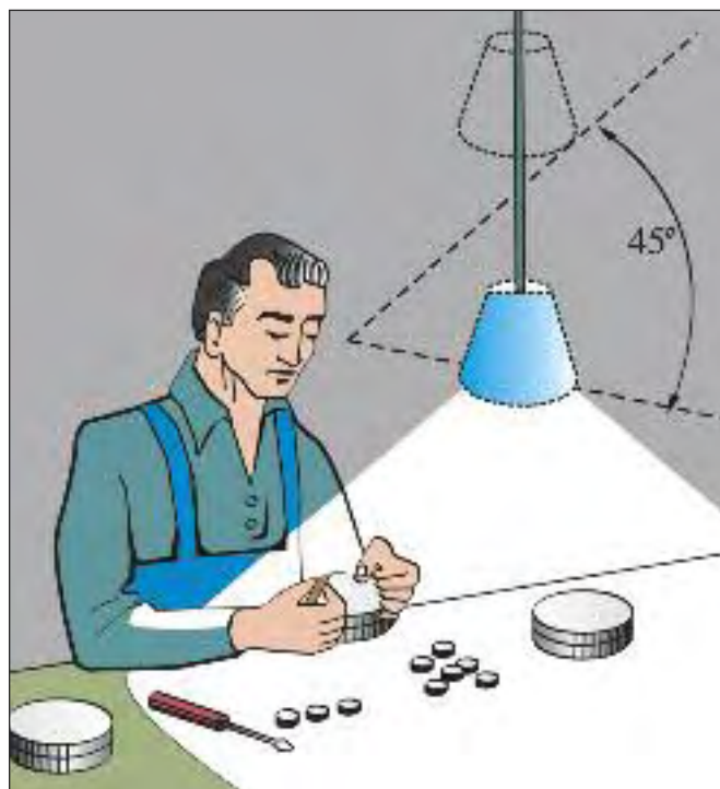
Figure 70a. A shaded lamp should be placed at the appropriate height.
