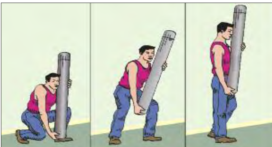
Figure 15b. A long heavy object can be lifted using the power of the legs by keeping the object as close to the body as possible.
