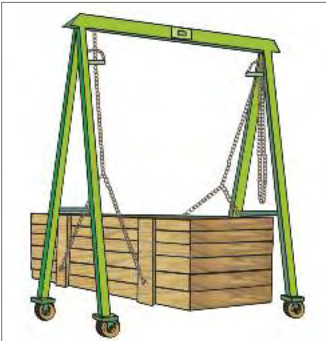
Figure 9a. A portable gantry is reliable, safe and easy to operate for carrying a heavy load a short distance with minimum elevation.
