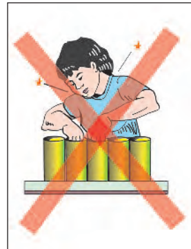
Figure 51b. For seated workers, worksurface height should be around elbow level.
