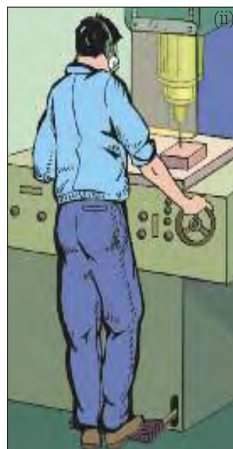
Figure 38a. (i) and (ii) Locate a foot pedal at floor level and make the pedal large enough for easy operation.
