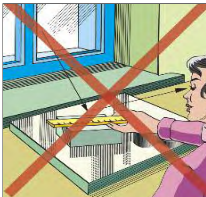
Figure 70d. Glare reflected from a polished surface.
