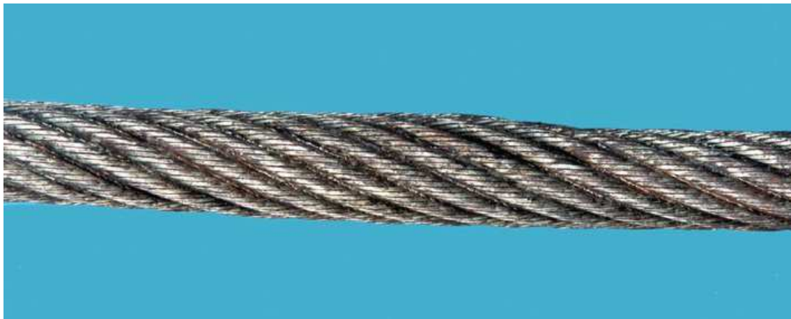
Figure B.15 — Local increase in rope diameter due to core distortion
