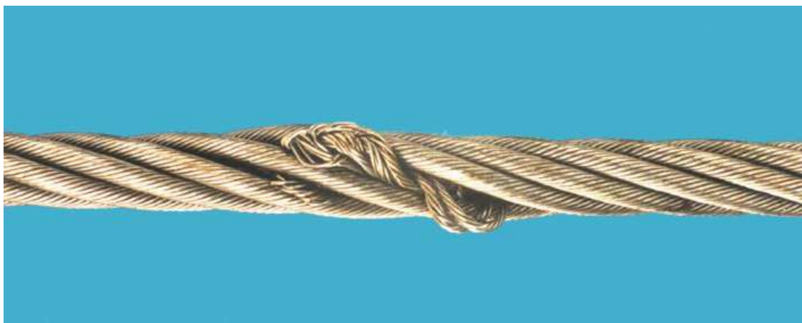
Figure B.11 — Core protrusion — Single-layer rope
