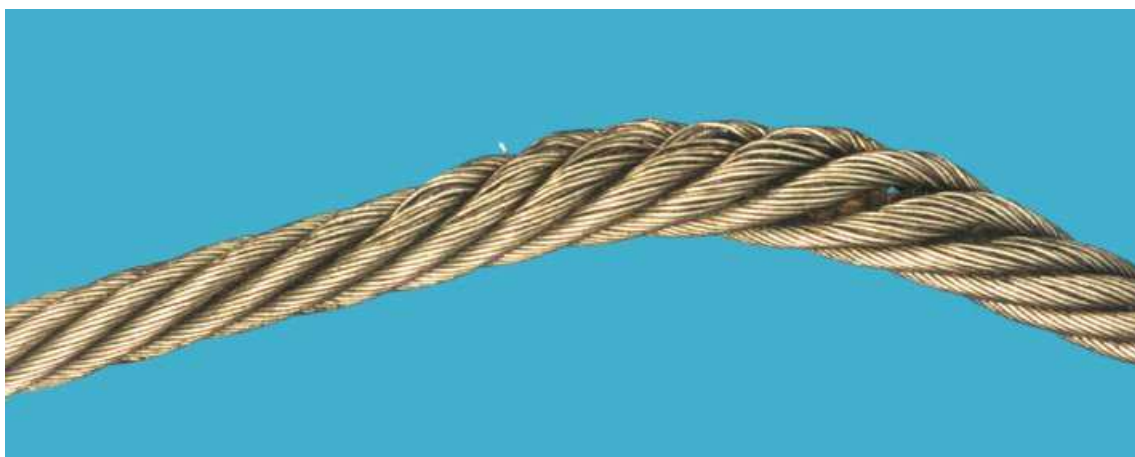
Figure B.16 — Flattened portion
