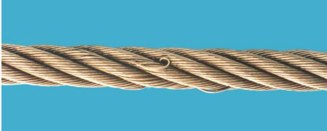
Figure B.14 — Wire protrusion
