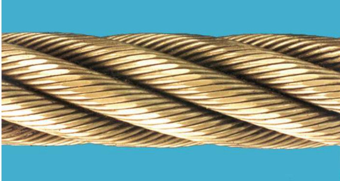
Figure B.1 — External wear
