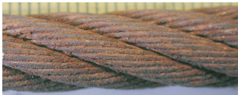
Figure I.2 — Wires rough to touch, general surface oxidation — Rating: 20 % towards discard
