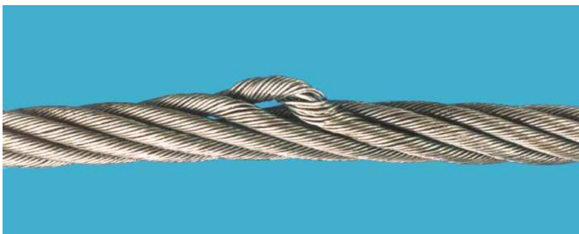
Figure B.13 — Strand protrusion/ distortion
