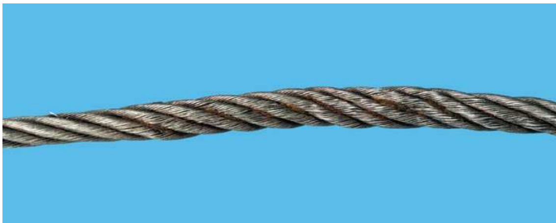
Figure B.17 — Flattened portion
