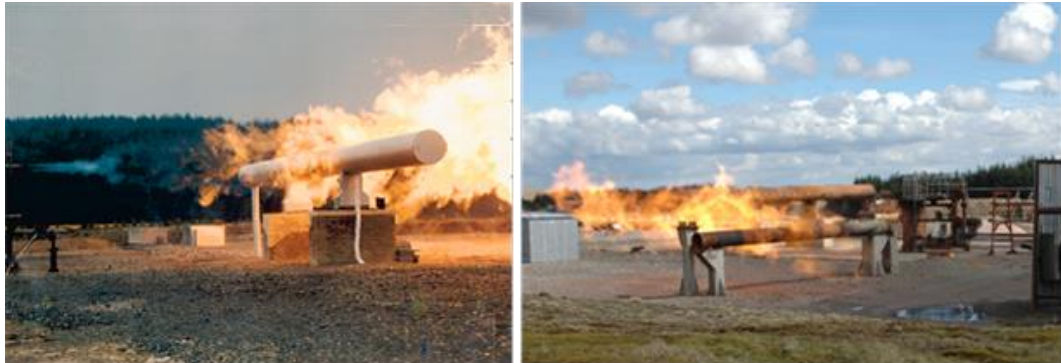
Figure 4: Natural gas jet fires impinging on a pipe
