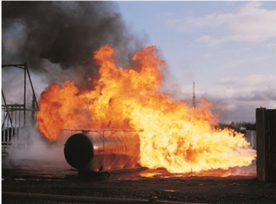
Figure 7: Propane jet fire impinging on a vessel
