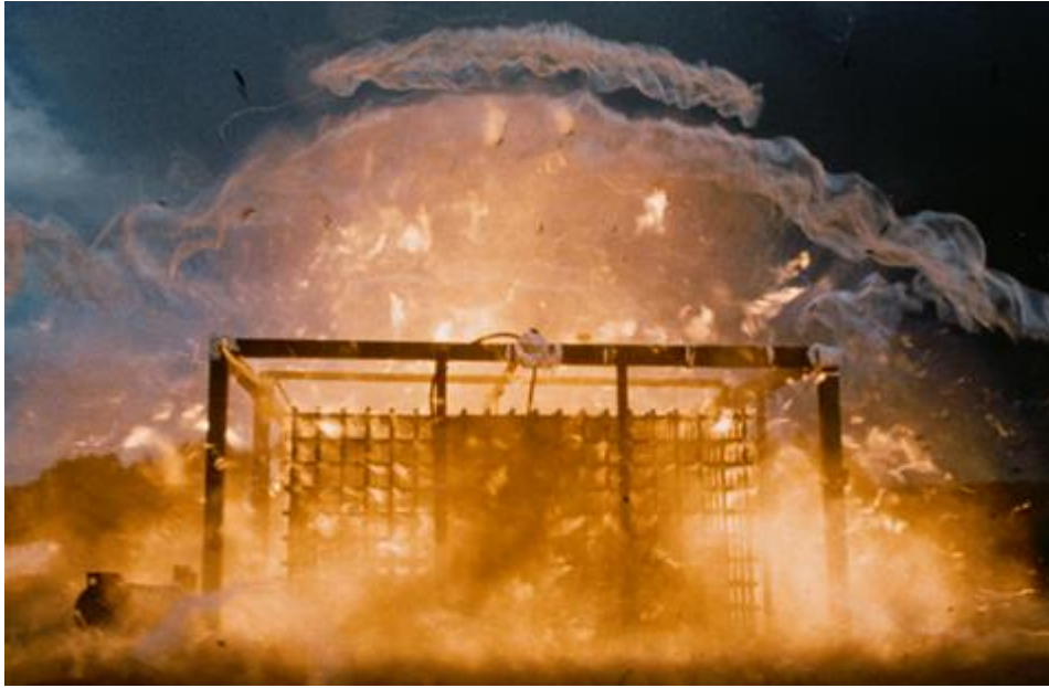
Figure 11: Deflagration experiment using idealised obstacle grid
