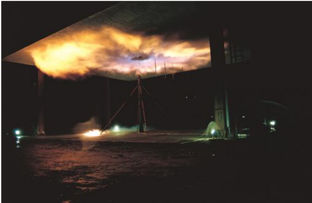
Figure 5: High pressure natural gas jet fire impacting on a roof
